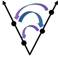
Figure 1: In the primal, the Sinkhorn algorithm alternately projects the iterate P = XKY \in \mathbb{R}^{n \times n} onto the two subspaces corresponding to the row/column marginal constraints. The Osborne algorithm is analogous, but with P = XKX^{-1} and n subspaces.
